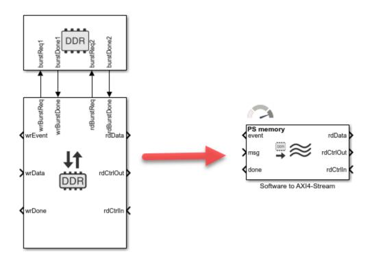
• AXI4 Random Access Memory - Use this block to replace a Memory Channel block with the **Channel type** parameter set to AXI4 Random Access connected to a Memory Controller block.
