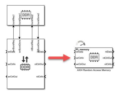
• AXI4 Video Frame Buffer - Use this block to replace a Memory Channel block with the **Channel type** parameter set to AXI4 Video Frame Buffer connected to a Memory Controller block.
